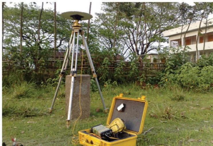
Setting coordinates for reference points in images using GPS technology
